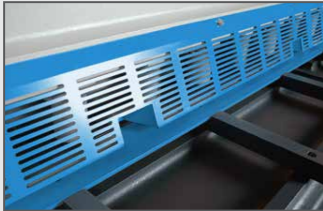
Hand safety guard with hand gaps for handling small sheets.
